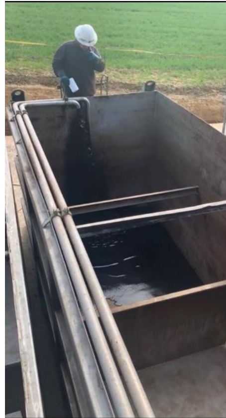
High quality crude oil produced during well test (33° API)
